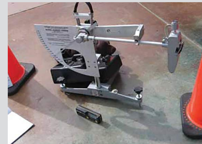
Pendulum test in progress
